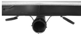
Black/Grey Tank Drain & Valves
