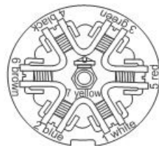
7-Way Trailer Plug- car end rear view
